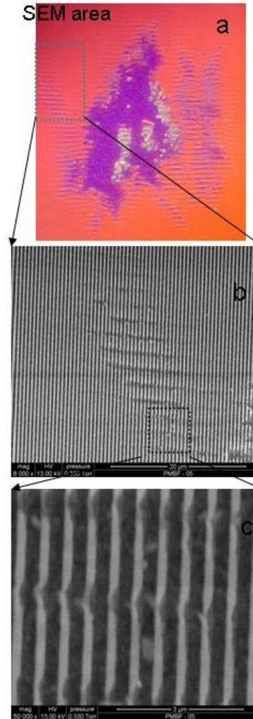
Fig. 3. Scanning Electrons micrography images of the damage sites with increasing scales (a-c). (a) The ripples of period  $2.5\ \mu\text{m}$  are visible near the main damage site. (b) They are perpendicular to the grating lines and (c) are responsible for the initiation damage. Incoming wave is coming from left to right.
