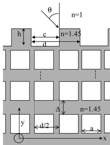
Fig. 1. Two-dimensional photonic crystal composed of silica (in gray, refractive index  $n=1.45$ ) and air (in white,  $n=1$ ). Air holes have a square cross section. The binary grating has grooves with height  $h$  and width  $c$  and presents a period denoted  $d$ .
