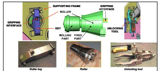
Fig. 7. Principal mechanical tools and roller parts.
