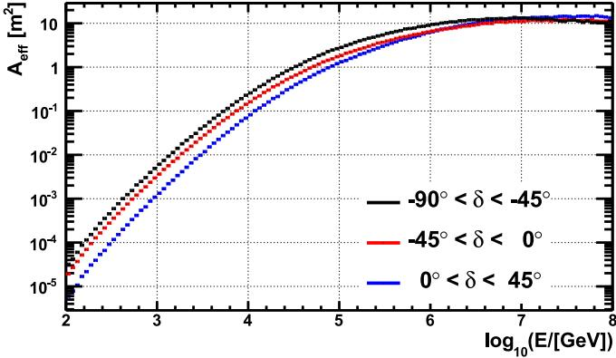
**Fig. 1.** Time-averaged muon-neutrino effective area of the ANTARES neutrino telescope as a function of energy for different declination bands  $\delta$  for the considered data-taking period. Typical quality cuts as derived in this analysis ( $\Lambda > -5.35$ ,  $\beta < 1^\circ$ ) are applied.
