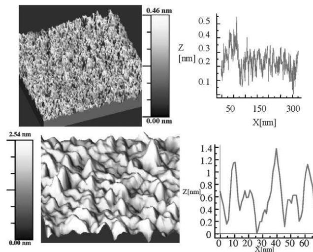
**Fig. 2** (Top) AFM image ( $400 \times 400$  nm) of grafted undecanoic acid on Si(100) wafer and topological profile, (down) AFM image ( $70 \times 70$  nm) of grafted  $\text{Mn}_{12}$  on Si(100) wafer and topological profile.
