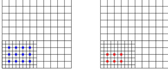
Figure 8: Restriction zone  $A_l$  on the left and correction zone  $\hat{A}_l$  on the right (e.g. for a 5-point stencil operator)
