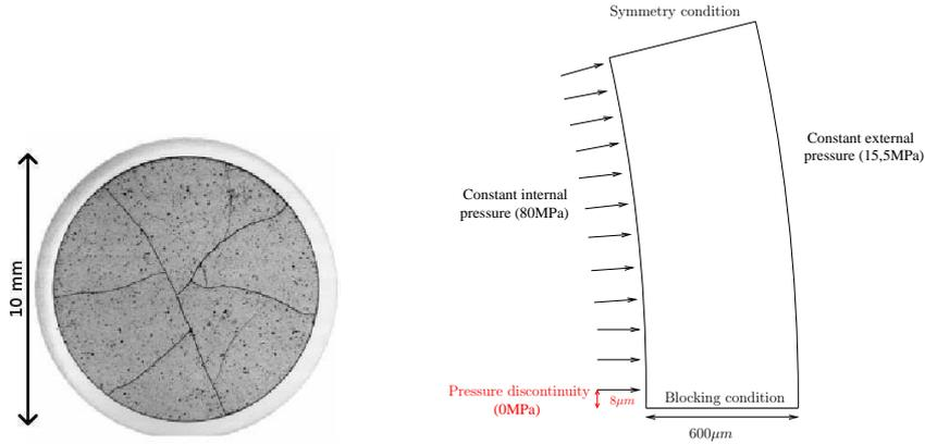
Figure 3: Problem definition - 2D plane strain test case
