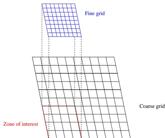
Figure 4: Example of hierarchical meshes used in a local multi-grid method
