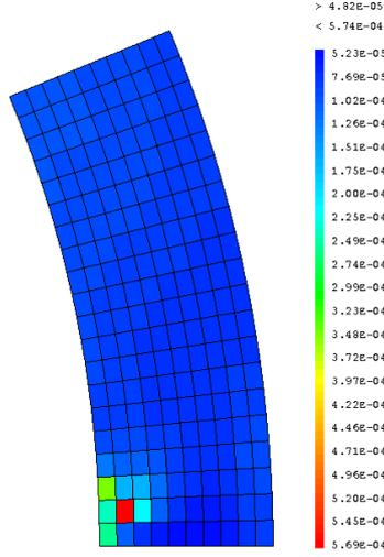
Figure 16: Local error given by the ZZ a posteriori error estimator - 2D plane strain test case
