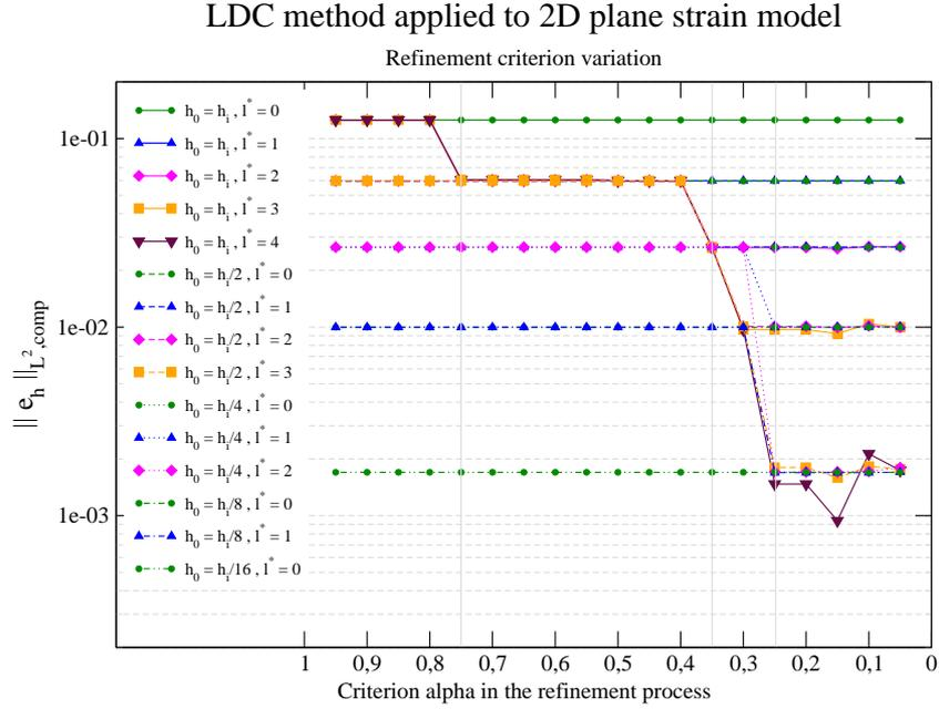
Figure 17: Composite  $L^2$  error norm according to the criterion  $\alpha$  used on the refinement process - 2D( $r, \theta$ ) test case
