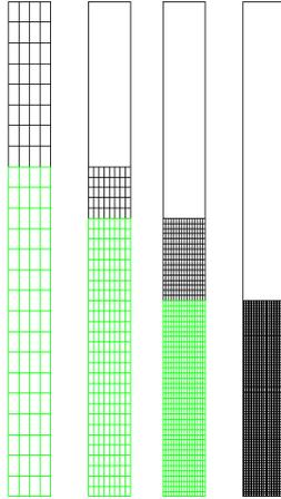
Figure 15: Example of nested meshes - A posteriori error estimation with  $\alpha = 0.15$  - 2D axisymmetric test case (current mesh in black, zone to refined in green) -  $h_0 = h_i$
