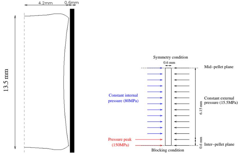
Figure 2: Problem definition - 2D axisymmetric test case
