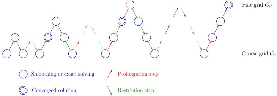
Figure 6: Representation of a local FMG process
