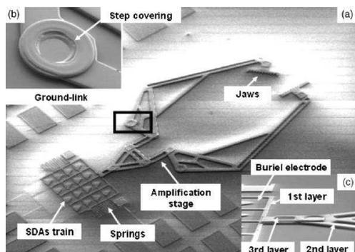
Fig. 1. Articular polysilicon micro-gripper developed at I.E.M.N. (C.N.R.S.) [51], and actuated by 16 Scratch Driven Actuators.
