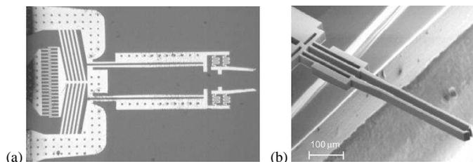
Fig. 5. (a) SOI compliant microgripper ( $1,200\ \mu\text{m} \times 900\ \mu\text{m} \times 50\ \mu\text{m}$ ) for insertion applications [43]; (b) SU-8-based microgripper (thin metal resistor patterned at the bottom of the structure) to operate in physiological ionic solution [24]
