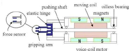
Fig. 2. Schematics of a superelastic NiTi flexure hinge microgripper (15.5 mm  $\times$  5.22 mm  $\times$  0.5 mm), actuated by 500 mN electromagnetic actuator, and including 44  $\mu\text{m}$ -thick PVDF force sensor at the gripper tip [40].
