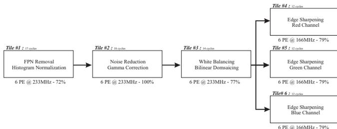
Fig. 3. Algorithms arrangement on the different computing tiles.
