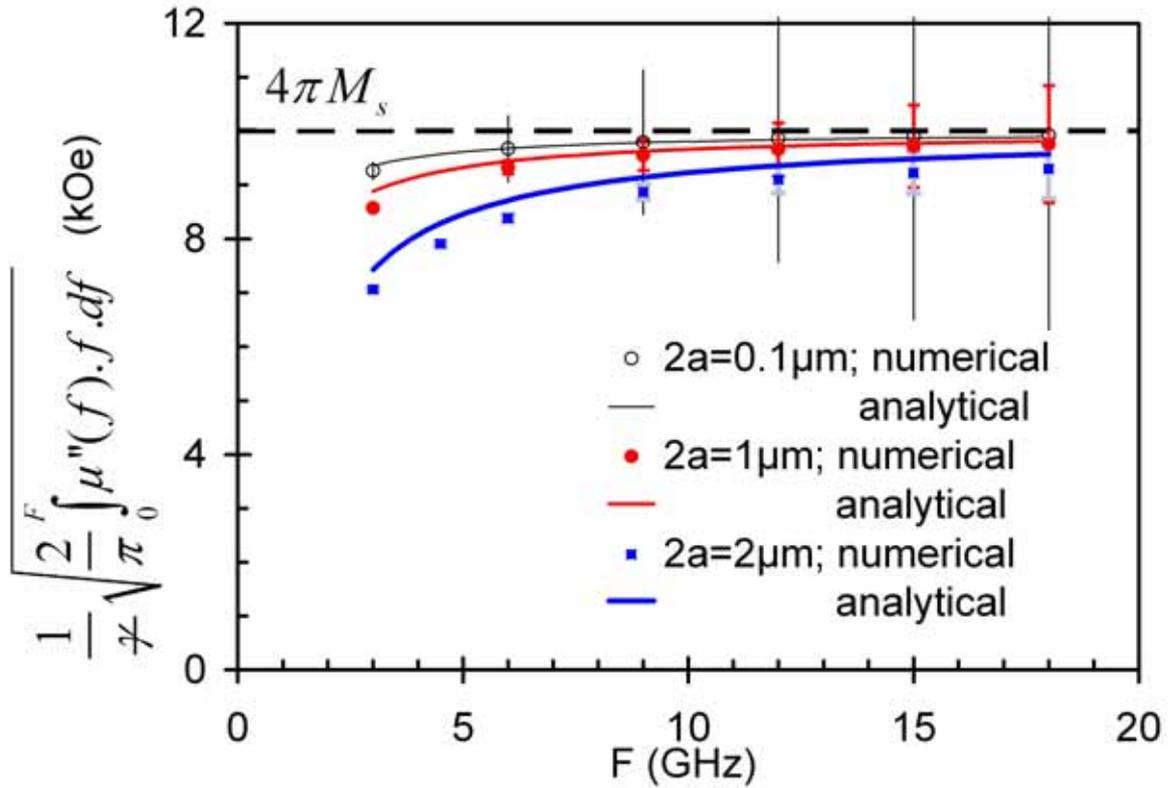
FIG 3. The efficient dynamic magnetization  $M_\mu(F)$  associated with the calculated permeabilities represented in Fig. 2, obtained either by numerical integration (symbols), or by analytical estimates (lines). The error bars represent typical experimental errors and the dashed line corresponds to the saturation magnetization.
