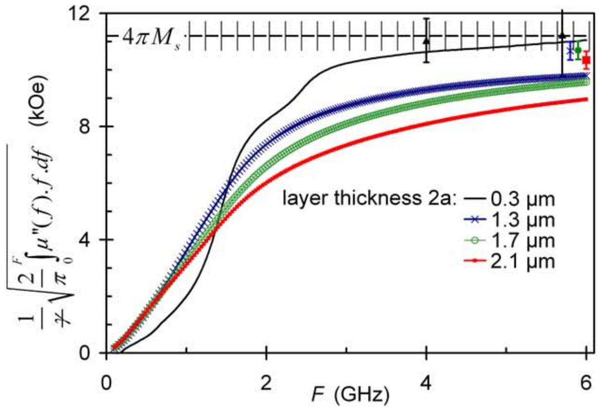
FIG. 5. The efficient dynamic magnetization  $M_\mu(F)$  associated with the measured permeabilities represented in Fig. 4, and a comparison with the saturation magnetization values (dashed line with error bars). The extrapolation of the saturation magnetization from  $M_\mu(F)$  using analytical estimates is also represented, with appropriate error bars.
