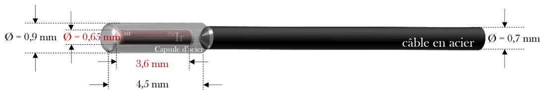
Figure 1. 17 : Source microSelectron HDD V2, Nucletron
