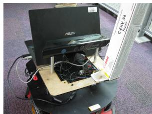
The pioneer 3 robot equipped for mapping experiments. On top of a long cardboard box, the magnetometer is protected from the metallic parts of the robot.
