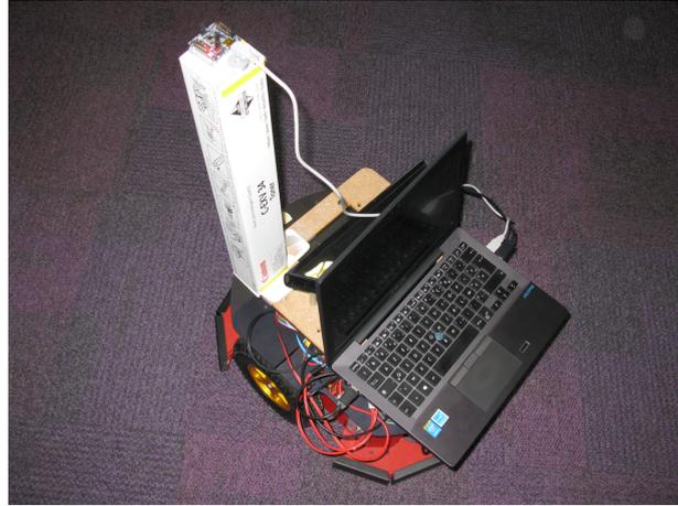
**Figure 6.4:** The pioneer 3 robot equipped with a Kinect 1 and MEMS magnetometer used for experiments. The magnetometer is mounted on top of a long cardboard box to avoid magnetic field disturbances due to metallic parts of the robot.
