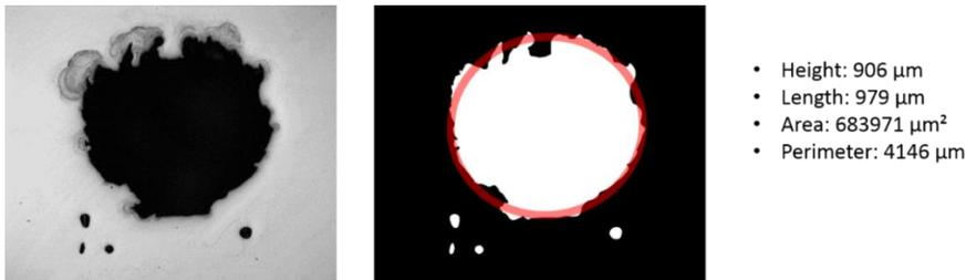
Figure 3: Image processing of a pore
