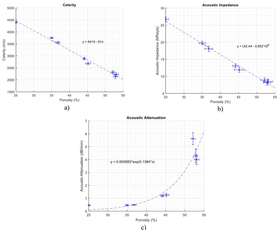
Figure 3: Acoustic properties of porous stainless steel as a function of the porosity. a) celerity of ultrasonic waves, b) acoustic impedance, c) acoustic attenuation.
