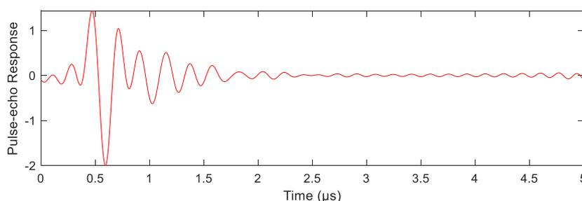
Figure 5: pulse-echo response of a transducer with a 25 % of porosity backing SSU02
