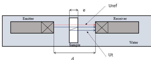
Figure 2: the principle of the insertion substitution method for the characterization of acoustic properties of materials
