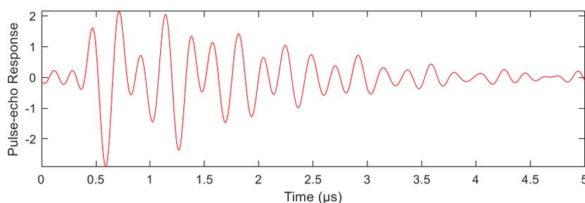
Figure 6: pulse-echo response of a transducer with a 45 % of porosity backing SSU25
