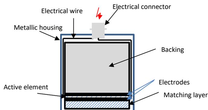
Figure 1: Schematic view of a transducer
