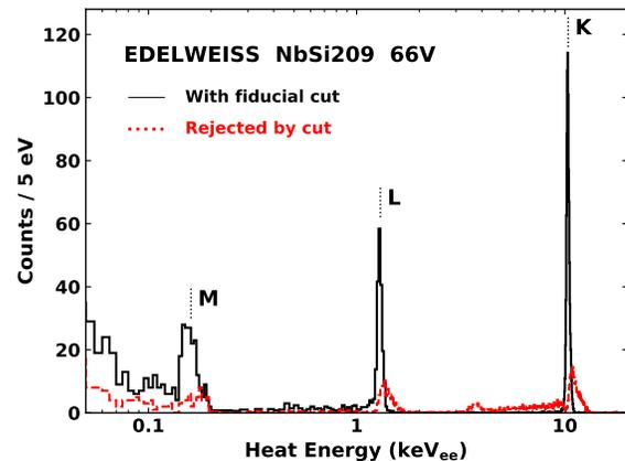
FIG. 2. Energy spectrum recorded at a bias of 66 V following the  $^{71}\text{Ge}$  emitted x-ray lines induced by the neutron activation of the Ge detector, resulting in the strong lines characteristic of  $^{71}\text{Ge}$  x-ray emissions. Black: events selected with the fiducial selection discussed in the text. Red: events rejected by the selection.
