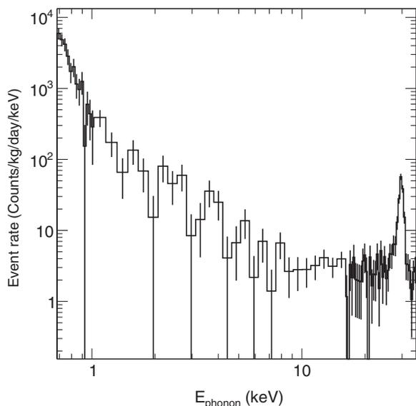
FIG. 4. Efficiency-corrected energy spectrum of the blinded part of the dataset after nominal analysis data selection and  $E_{ion} > 400$  eV criterion (corresponding to the efficiency curve in dark green in Fig. 3).
