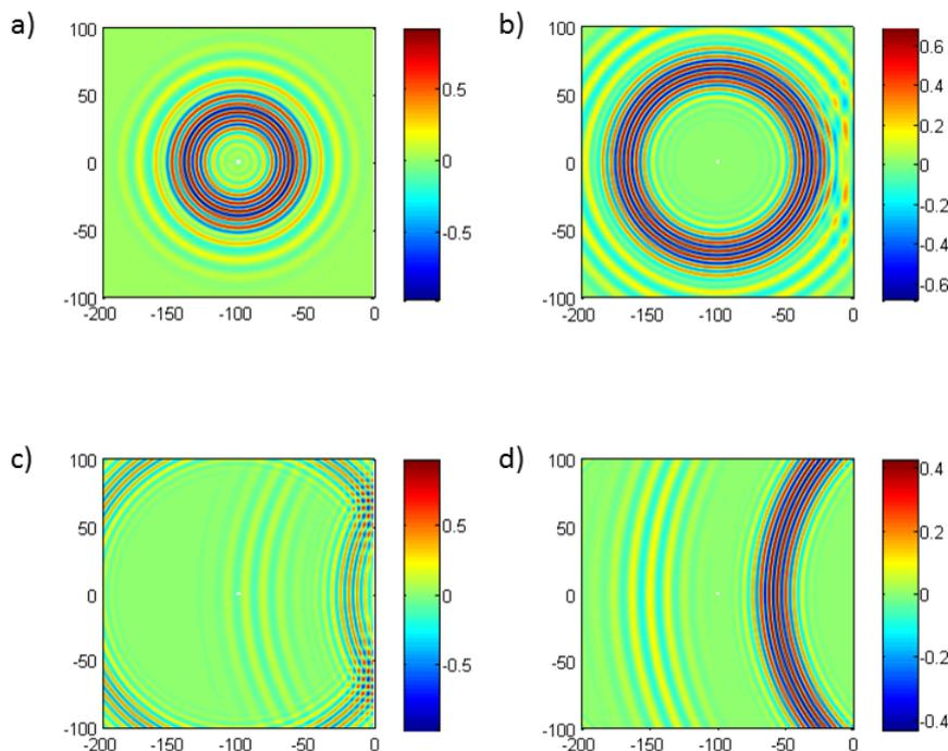
**Figure 9.** Four snapshots of the normal displacement associated to guided wave propagation in a plate with account of edge reflection (a) at  $18\mu s$ , (b) at  $31\mu s$ , (c) at  $54\mu s$ , and (d) at  $72\mu s$ .
