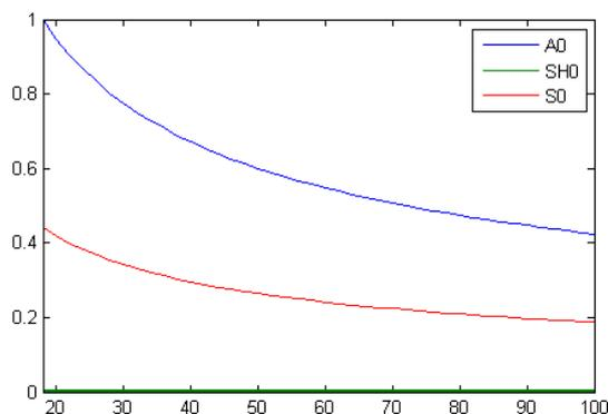
**Figure 8.** Normalized normal modal displacement along an axis from a distance of  $\lambda_{max}$  of the edge of the source centered at  $(0, 0)$ .
