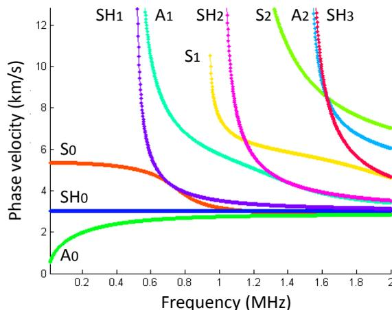
**Figure 7.** Dispersion curves of a 3-mm-thick aluminium plate.
