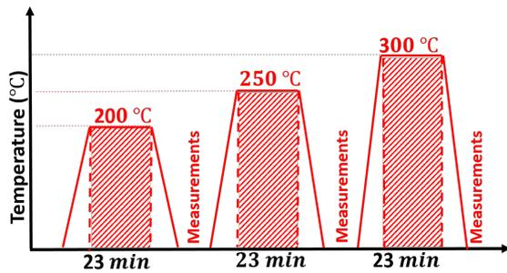
Figure 3: Annealing procedure.
