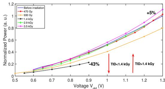
**Figure 7:** Power degradation at different TID levels.
