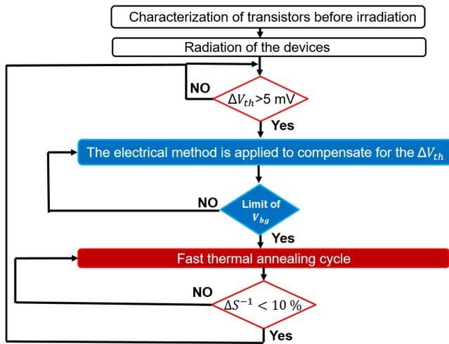
Figure 8: Flow diagram of the mixed hardening methodology.
