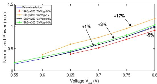
Figure 10: Power recovery after applying the T- $V_{bg}$  method.
