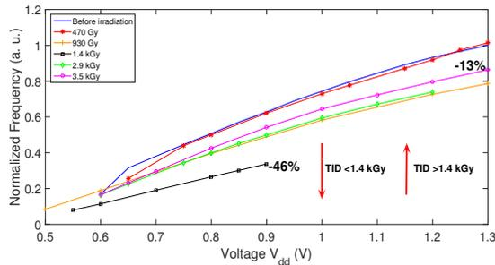
**Figure 6:** Frequency degradation at different TID levels.
