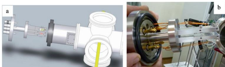
Fig. 5: Views of the specific double-diode intensity monitors: drawing (a) and picture (b).
