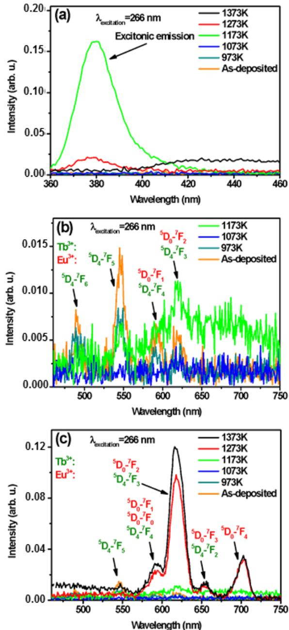
**Figure 9.** PL spectra of ZnO:Tb (1.6 at.%), Eu (1.3 at.%) film for a laser excitation at 266 nm, in the spectral range (a) from 360 to 460 nm and (b) from 460 to 750 nm for the lower annealing temperatures and (c) for all  $T_A$ .
