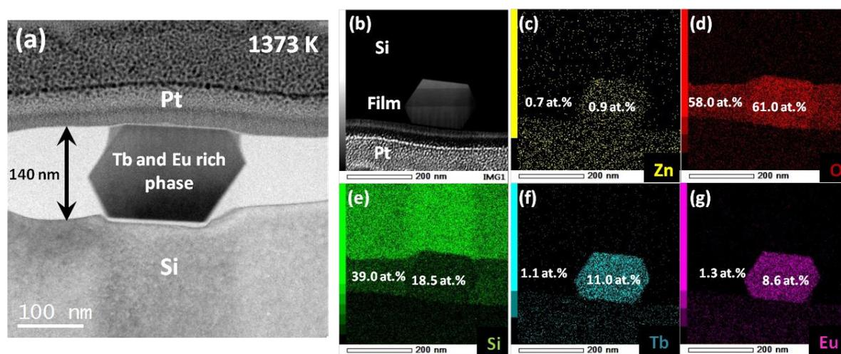
**Figure 6.** (a) Bright field TEM image for the ZnO:Tb,Eu film for  $T_A = 1373$  K. (c-g) Chemical maps of Zn (c), O (d), Si (e), Tb (f) and Eu (g), corresponding to the STEM HAADF image in figure (b).
