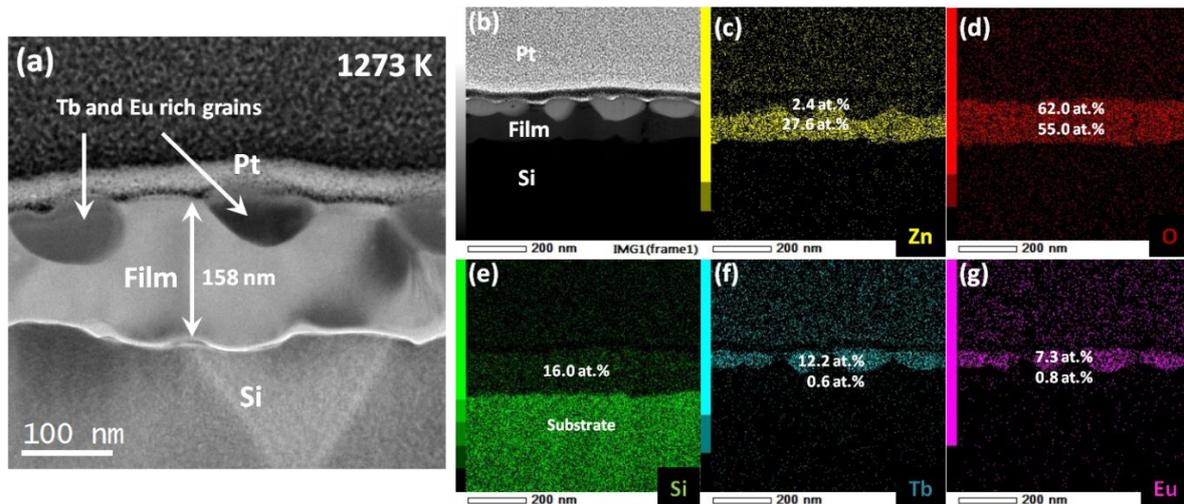
**Figure 4.** (a) Bright field TEM Image of the ZnO:Tb,Eu film for  $T_R = 1273 \text{ K}$ . (c-g) Chemical maps of Zn (c), O (d), Si (e), Tb (f) and Eu (g), corresponding to the STEM HAADF image in figure (b).
