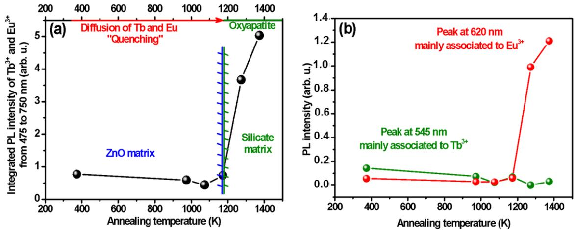
**Figure 10.** (a) Plot of integrated PL from 475 to 750 nm and (b) emission intensities at 545 nm and 620 nm versus  $T_A^\circ$  based on the PL spectra in figures 9(b and c) for an excitation at 266 nm.
