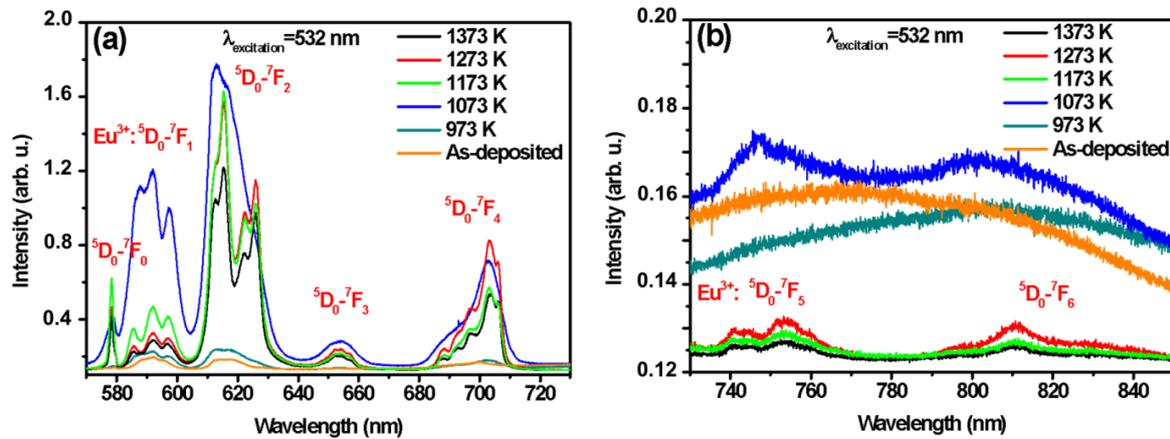
**Figure 11.** PL spectra from 570 nm to 730 nm (a) and from 730 nm to 850 nm (b) of ZnO:Tb,Eu films annealed at various  $T_A^\circ$  for a laser excitation at 532 nm.
