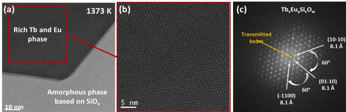
**Figure 7.** (a) HRTEM image of the ZnO:Tb,Eu film for  $T^\circ_A = 1373 \text{ K}$ . (b) HRTEM Image from the squared region in red of the grain in figure (a). (c) Fast Fourier Transform associated to the grain in figure (b).
