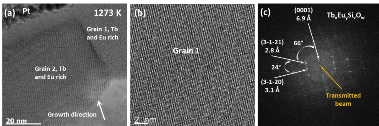
**Figure 5.** (a) Bright field TEM image of the ZnO:Tb,Eu film annealed at 1273 K showing two grains of a Tb and Eu rich phase localized at the upper part of the film. (b) HRTEM Image of grain 1, identified in figure 5(a). (c) Fast Fourier Transform of grain 1.
