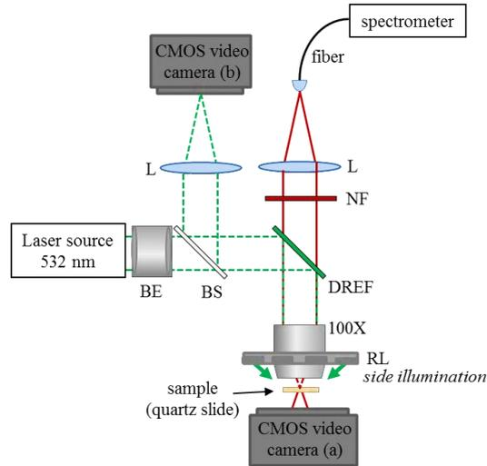
Figure 1 Schematic of the experimental setup. Abbreviations: BE: beam expander (x5), BS: beam splitter, DREF: dichroic razor-edge filter, 100X: microscope objective, NA = 0.8, RL: Ring LED, NF: Notch filter, L: achromatic lens. Video camera (a) enables lensless
