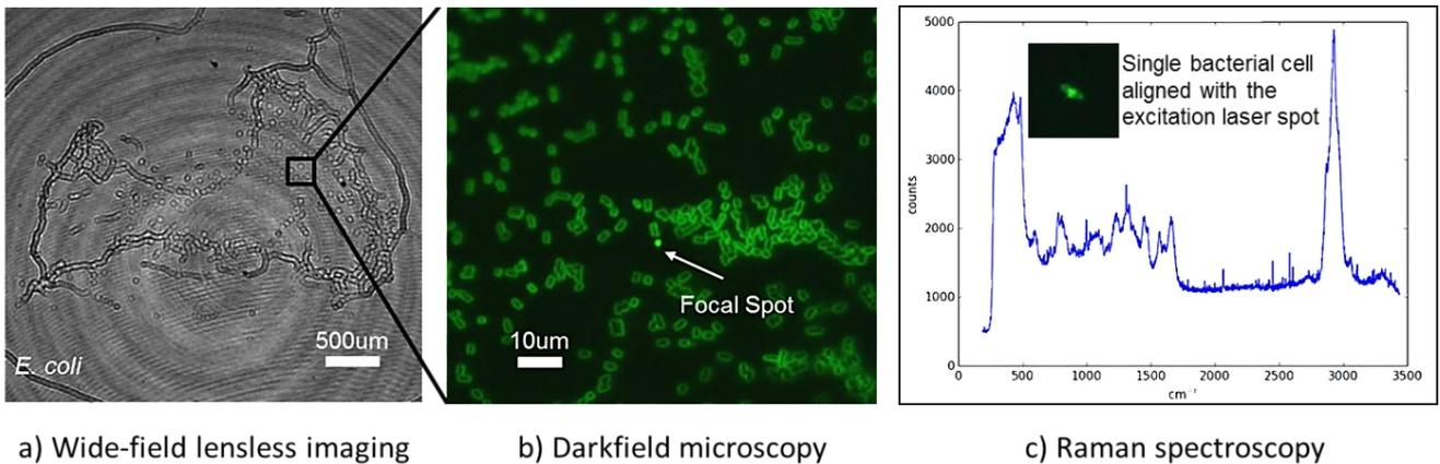
Figure 2 Illustration of the operation steps for a 1uL droplet with *E. coli* bacteria: a) lensless image giving a wide-field of view of the droplet evaporated onto the quartz substrate, and facilitating the selection of region of interest (square). b) standard microscope image of the bacteria and the laser spot to assist in accurate targeting, and c) typical Raman spectrum obtained on a single bacteria with 10s acquisition time.
