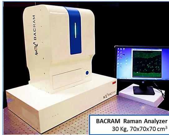
Figure 3 Photograph of the complete integrated Raman analyzer BACRAM
