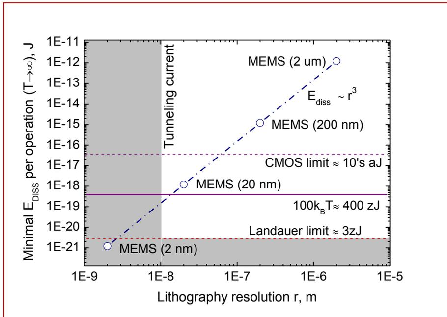
**Figure 10.** Simulated minimal dissipated energy trend  $E_{diss}$  for the ramping time tends to infinity according to lithography resolution  $r$  for device operated with four-phase PC's. Here we assume that  $L_{gap} = r/2$ .
