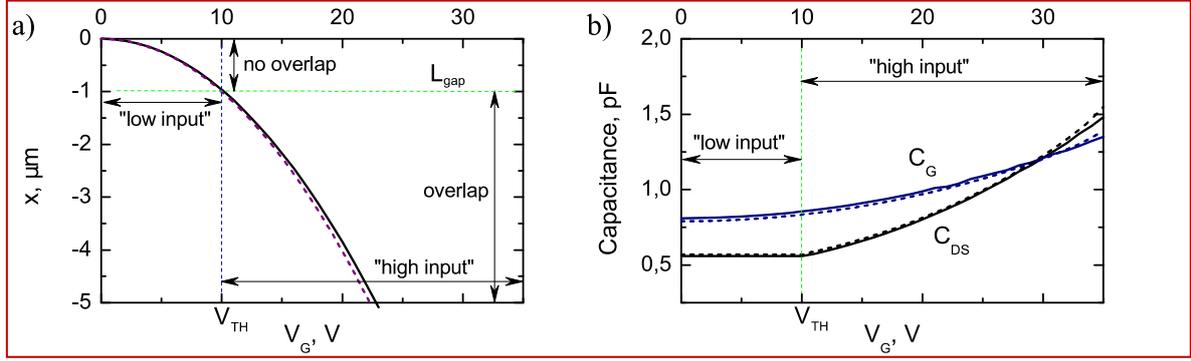
**Figure 6.** a) Moving mass displacement as a function of the input voltage  $V_G$ . b) Input  $C_G$  and output  $C_{DS}$  capacitances as a function of the input voltage  $V_G$ . Verilog-A model and MEMS+® simulation results are drawn as solid and dashed lines, respectively.
