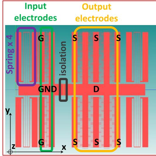
**Figure 5.** Top view of the contactless four-terminal MEMS element. Length of the structure is 1.2 mm, width is 1 mm, number of input fingers  $N_{in}$  is 110, number of output fingers  $N_{out}$  is 220.
