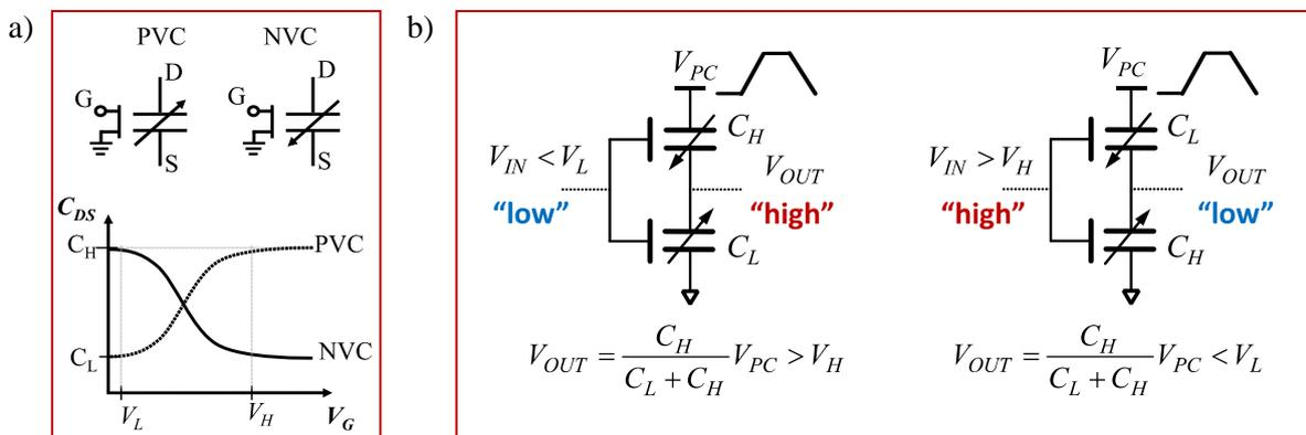
**Figure 2.** a) Capacitance–voltage (CV) characteristics and symbols for positive variable (PVC, dotted line) and negative variable (NVC, solid line) capacitors. The low and high voltage levels are denoted as  $V_L$  and  $V_H$ , respectively. The same notation ( $C_L$  and  $C_H$ ) is used for capacitance levels. b) Electrical schematics of simple CAL inverter circuit and cascading conditions.
