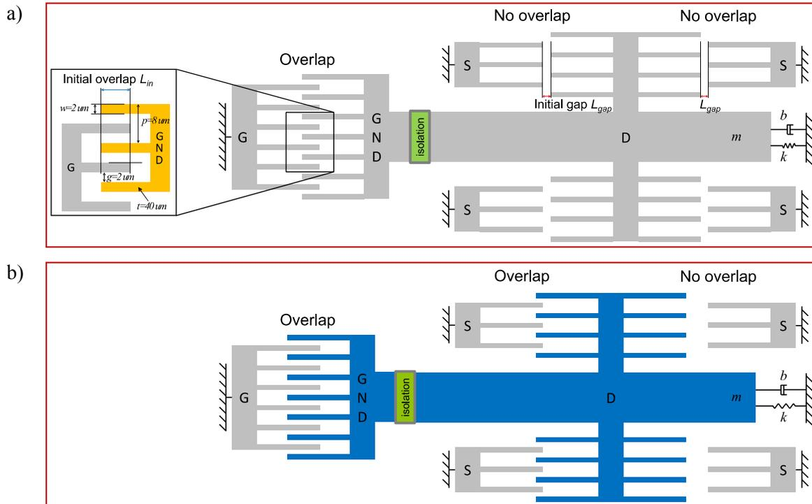
**Figure 4.** Two states of MEMS element as function of the moving mass displacement  $x$ . a) Low state:  $-L_{gap} \leq x \leq L_{gap}$ . Parameters of the comb-drive actuator are presented in the insert. b) High state:  $x < -L_{gap}$ .
