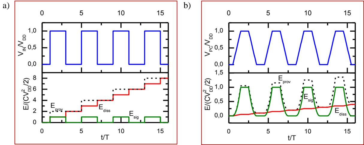
**Figure 1.** a) Static CMOS logic ( $RC \ll T$ ). Normalized input voltage  $V_{IN}/V_{DD}$  (first graph), normalized provided  $E_{prov}$ , dissipated  $E_{diss}$ , and signal energy  $E_{sig}$  (second graph). b) Adiabatic CMOS logic. Normalized power supply voltage  $V_{PC}/V_{DD}$  (first graph), normalized provided  $E_{prov}$ , dissipated  $E_{diss}$ , and signal energy  $E_{sig}$  (second graph).
