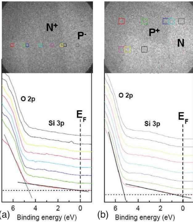
**Figure 5.** Top of the valence band spectra extracted from the same areas of interest as for the Si 2p core level spectra of figures 3 and 4. (a) N<sup>+</sup>/P<sup>-</sup>. (b) P<sup>+</sup>/N. The densities of states due to the O 2p and Si 3p orbitals are marked, together with examples of linear extrapolation in order to determine the valence band onsets. The threshold images with the relevant AOIs are reproduced for convenience.
