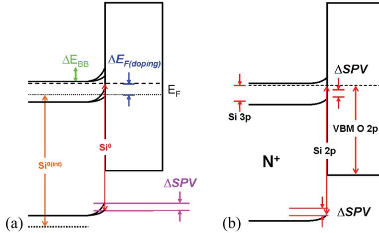
**Figure 6.** (a) Schema showing how doping, band bending and surface photovoltage interact to modify the electronic energy levels in  $N^+$  zones of  $N^+/P^-$  with respect to the values obtained for intrinsic silicon. The dotted lines represent intrinsic silicon; the dashed line is the position of the Fermi level in the heavily doped region. (b) Scale drawing of results for the  $N^+$  region in  $N^+/P^-$ , with the calculated SPV effect.
