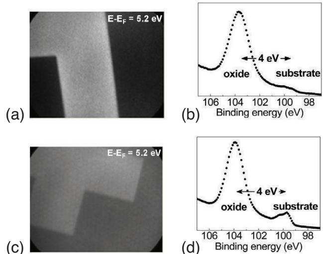
**Figure 2.** (a) and (c) Threshold images of  $\text{N}^+/\text{P}^-$  and  $\text{P}^+/\text{N}$ , respectively, using a 25  $\mu\text{m}$  field of view; (b) and (d) Si 2p spectra averaged over the field of view of (a) and (c), showing broad peaks given the energy resolution. The threshold images have been obtained using high resolution  $1 \times 1$  binning.
