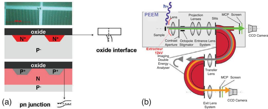
**Figure 1.** (a) Top: optical micrograph of doped patterns. Middle: N<sup>+</sup>/P<sup>-</sup> sample. Bottom: P<sup>+</sup>/N sample. Also shown: expected band line-ups in  $x$ - $y$  (pn junction) and  $z$  (oxide/substrate interface). (b) Schema of the XPEEM instrument used showing the direct PEEM, selected-area XPS and energy-filtered PEEM modes. The double hemispherical analyser suppresses the  $\alpha^2$  aberrations inherent in a single hemispherical analyser.
