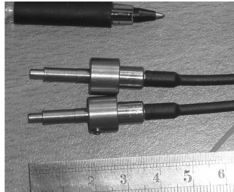
Figure 4. FBG contact pressure and temperature sensor.
