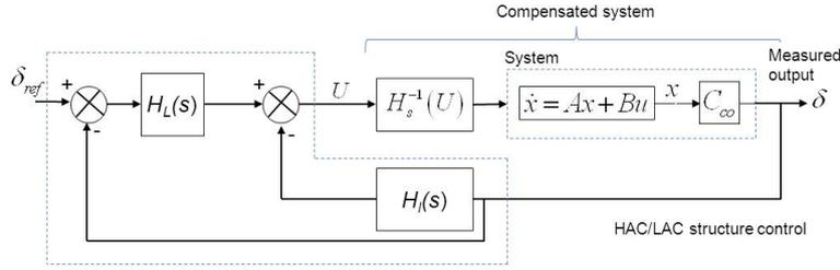
Figure 19: Scheme control of the cascaded HAC/LAC loops.
