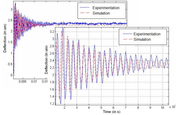
Figure 8: Experimental transient response for the  $\frac{\delta}{u}$  transfer operator ( $\delta$  in  $\mu m$  and  $u$  in Volt) and corresponding identified response.
