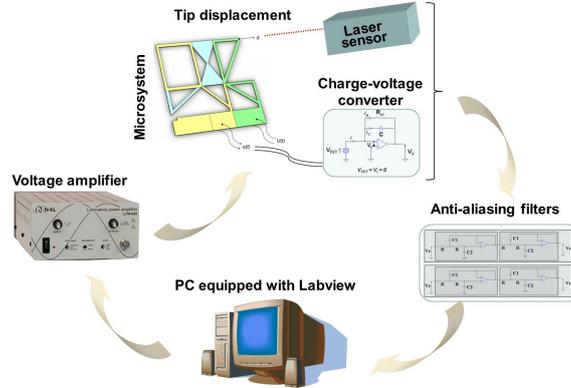
Figure 6: Schematics of the experimental setup.
