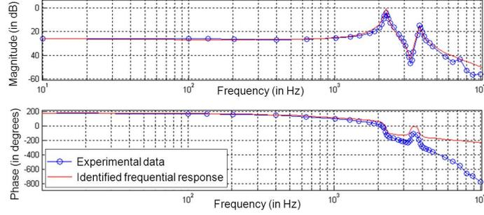
Figure 7: Experimental Bode diagram of the  $\frac{\delta}{u}$  transfer function ( $\delta$  in  $\mu m$  and  $u$  in Volt) and corresponding identified transfer function.
