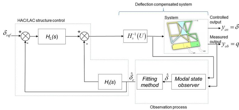
Figure 23: Complete observation/control scheme based on proprioceptive measurement.
