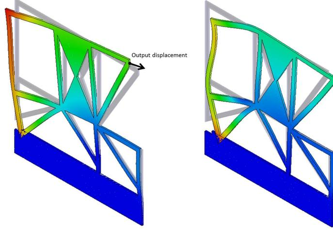
Figure 13: Mode shape plots of the pseudo-optimal structure associated with  $\omega_{n_1}$  on the left and  $\omega_{n_2}$  on the right. (Actuation and sensing parts within the structure are reported in Fig. 3.)
