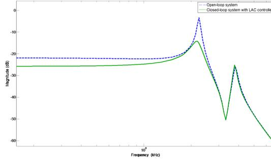
Figure 20: Bode diagrams in magnitude of the open-loop transfer  $\delta(s)/u(s)$  and pre-compensated closed-loop transfer with  $H_L(s)$ .
