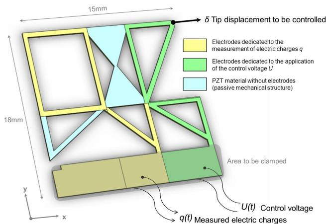
Figure 3: 3D CAD of the left-finger PZT microactuator with integrated sensing capabilities.
