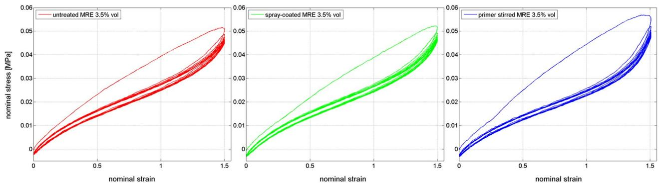
**Fig. 17** Stress-strain response of the MRE samples with a particle volume fraction of 3.5 % during cyclic loading parallel to particle alignment at a strain rate of  $0.02 \text{ s}^{-1}$ : **a** untreated MRE, **b** spray-coated MRE, and **c** primer stirred MRE
