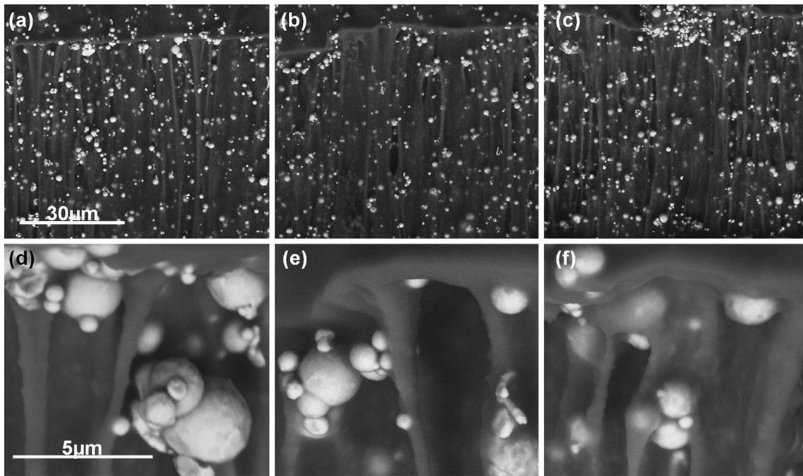
**Fig. 15** SEM micrographs (1,500×) of the interfacial adhesion between the iron fillers and the silicone matrix at a strain of 140 % in MRE samples with a particle volume fraction of 30 %: **a** untreated
