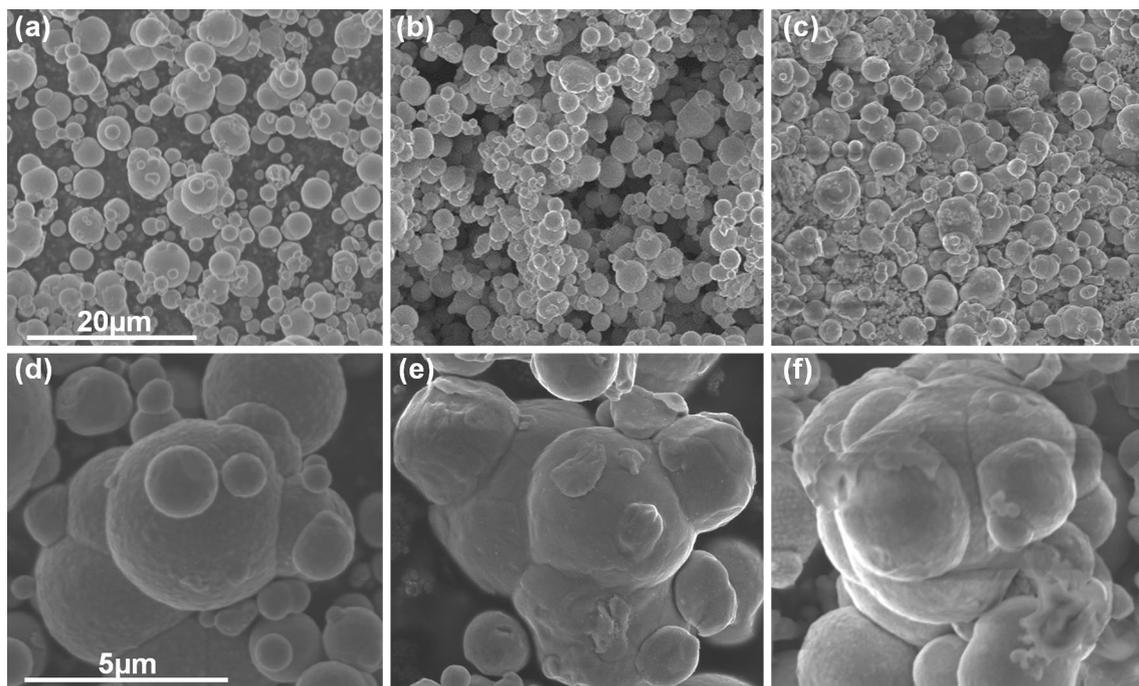
**Fig. 10** SEM micrographs (1,500 $\times$ ) of the carbonyl iron particles with a median particle size of 3.5  $\mu\text{m}$ : **a** untreated particles, **b** spray-coated particles, and **c** primer stirred particles; SEM micrographs
