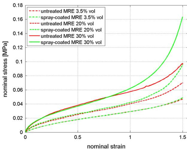
**Fig. 21** Influence of the primer treatment at high strain: stable upload curves for the spray-coated MREs compared to the untreated MREs for particle volume fractions of 3.5, 20 and 30 %
