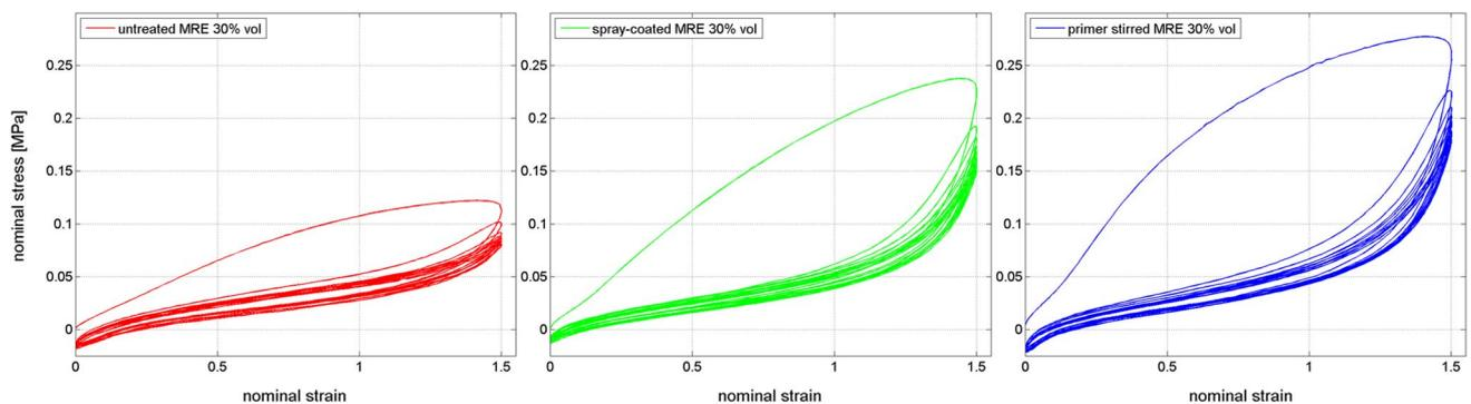
**Fig. 18** Stress-strain response of the MRE samples with a particle volume fraction of 30 % during cyclic loading parallel to particle alignment at a strain rate of  $0.02 \text{ s}^{-1}$ : **a** untreated MRE, **b** spray-coated MRE, and **c** primer stirred MRE
