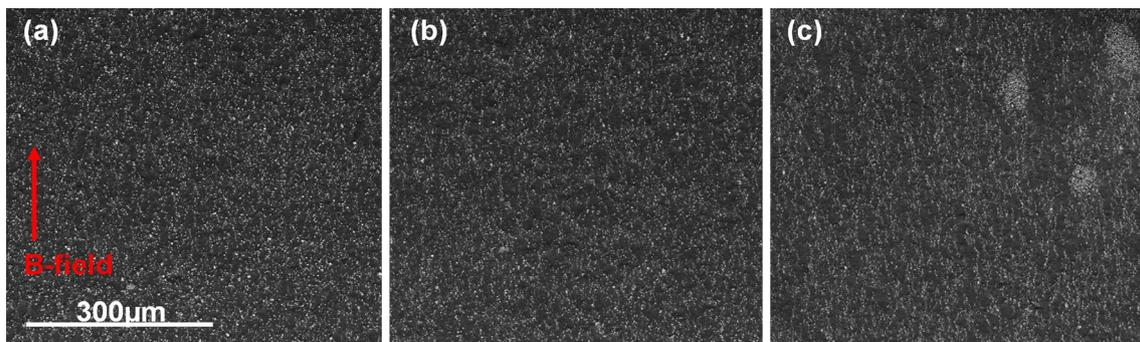
**Fig. 12** SEM micrographs (200×) of particle chain alignment in MRE samples with a particle volume fraction of 30 %: **a** untreated MRE, **b** spray-coated MRE, and **c** primer stirred MRE. The *arrow* indicates the direction of the magnetic field during curing
