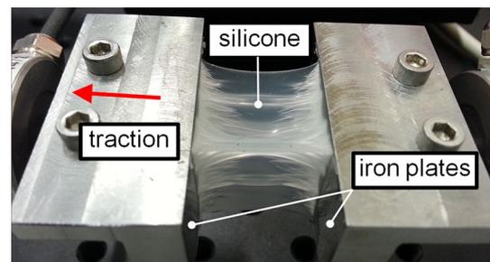
**Fig. 8** Image of the traction test of the silicone cast between two primer treated iron plates in the deformed state
