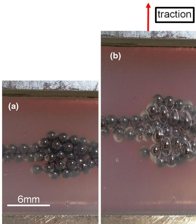
**Fig. 7** Preliminary macroscopic test: **a** 1.5 mm steel spheres cast in the silicone matrix at the unstrained state; **b** debonding between spheres and silicone matrix under traction at 40 % nominal strain
