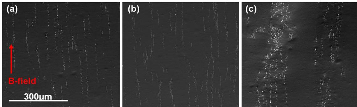
**Fig. 11** SEM micrographs (200×) of particle chain alignment in MRE samples with a particle volume fraction of 3.5 %: **a** untreated MRE, **b** spray-coated MRE, and **c** primer stirred MRE. The *arrow* indicates the direction of the magnetic field during curing
