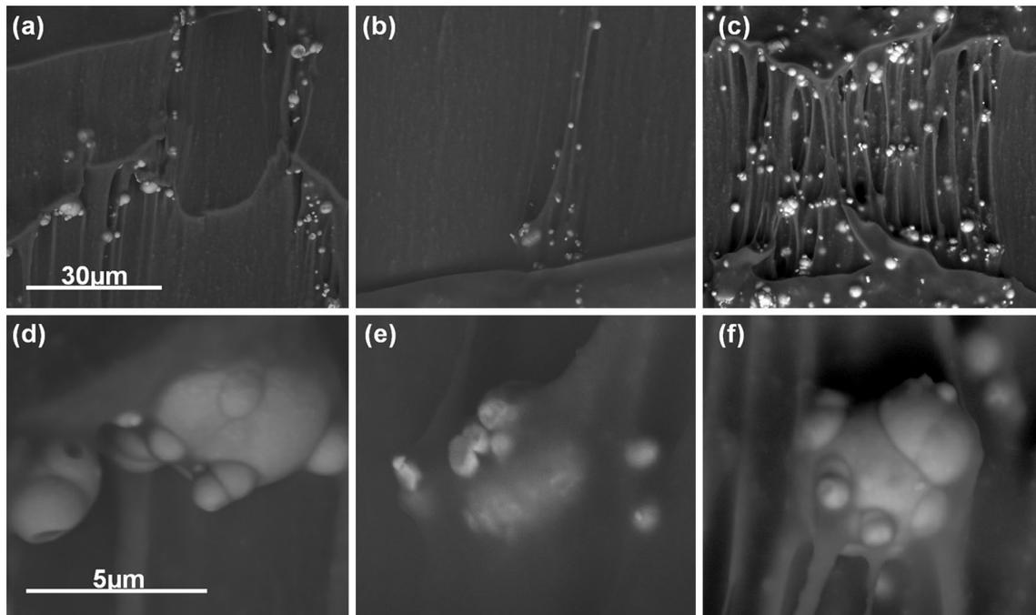
**Fig. 14** SEM micrographs (1,500 $\times$ ) of the interfacial adhesion between the iron fillers and the silicone matrix at a strain of 140 % in MRE samples with a particle volume fraction of 3.5 %: **a** untreated
