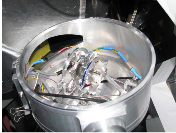
Figure 3.2: Photography of the Köln plunger device placed in the target chamber
