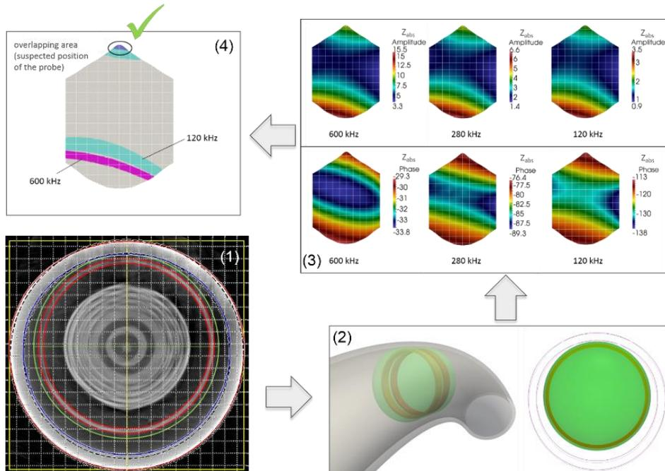
**Figure 4.** X-ray imaging of the probe at the top of the bending (1), corresponding geometric modelling (2), phase and amplitude of the simulated signal for the admissible positions of the probe (here operated in absolute mode) (3), and intersection of the reduced envelopes (4).
