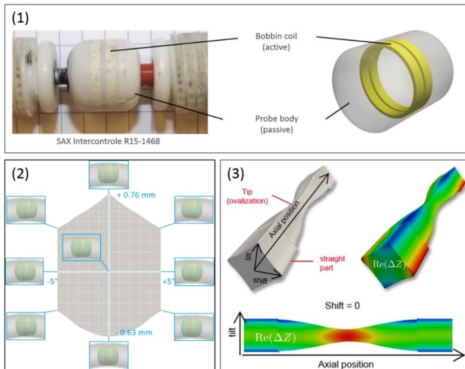
**Figure 2.** Geometric modelling of the plastic body of the probe (1), 2D envelope of the admissible positions of the probe at a given axial position in the bending (2), 3D envelope for the complete U-bend tube and corresponding impedance variation of the signal (3).
