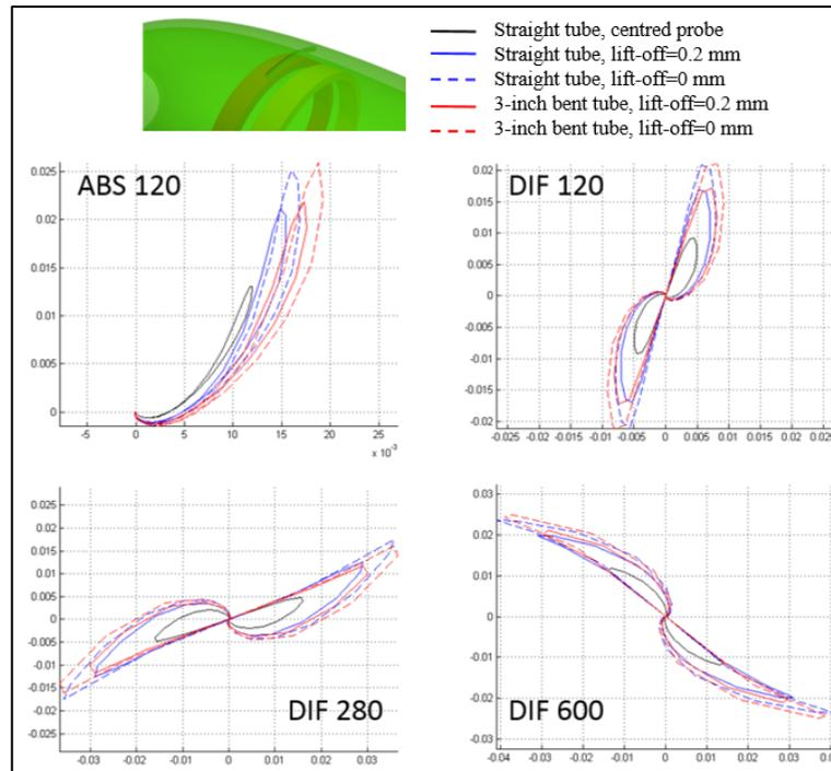
**Figure 6.** Simulation of the ECT signal with a circumferential notch (40% depth, 6 mm x 0.15 mm) and two bobbin coils operated in absolute mode (ABS) at 120 kHz and differential mode (DIF) at 120, 280, 600 kHz.
