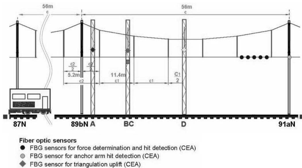
Figure 1. Control gate installed in Switzerland (Lötschberg), including several FBG sensors and remote FBG measurement systems.
