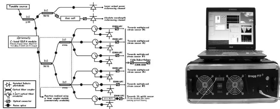
Figure 3. BraggFit<sup>3</sup> monitoring system architecture and picture.
