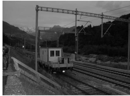
Figure 6. FBG measurement units in the container to control any train passing the control gate.
