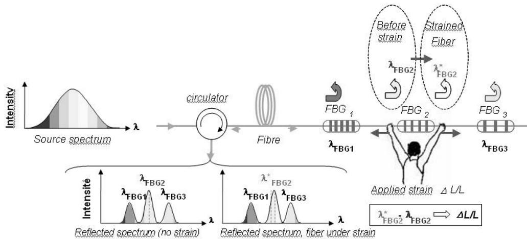
Figure 2. FBG principle: the spectral effect of strain on Bragg wavelength.
