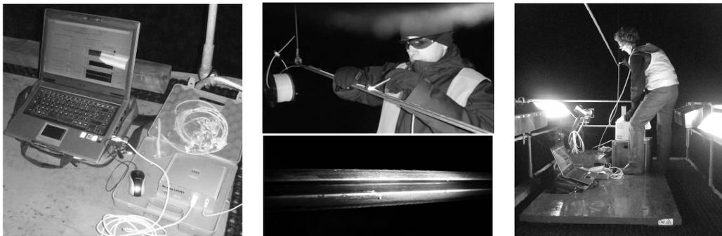
Figure 5. *BraggLight* unit used for real-time control of FBG line epoxy curing on contact wire.
