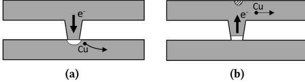
**Figure 3: Voiding in via-metal structures: (a) downstream via, and (b) upstream via**
