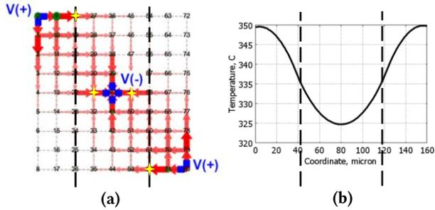
**Figure 5: Current distribution in the grid (as depicted by arrows), (a); non-uniform temperature distribution along the horizontal rails, (b). Dashed lines show borders of poly-heaters. Four possible early voiding locations are shown in (a).**
