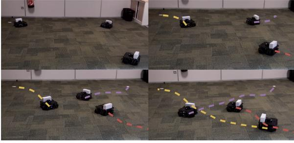
Fig. 5: Experiment with three Turtlebots 3. From left to right, top to bottom.
