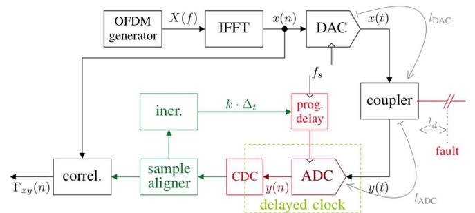
Fig. 4. Schematic diagram of an OMTDR based cable diagnosis system using a correlator between the injected signal  $x(n)$  and the received signal  $y(n)$  to detect the location of the fault. The acquisition resolution is improved through a pseudo oversampling achieved using a constant phase-shift increasing on the sampling clock of the ADC.
