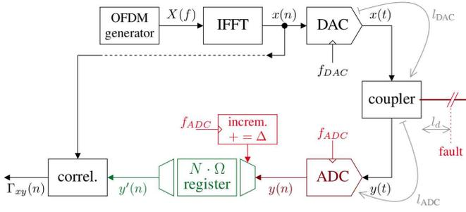
Fig. 5. Schematic diagram of a cable diagnosis system using a correlator between the injected signal  $x(n)$  and the received signal  $y(n)$  to detect the location of the fault. Acquisition resolution is improved through the reconstruction of the received signal which is sampled at  $f_{ADC}$ , a slightly different clock frequency than that of the DAC  $f_{DAC}$ .
