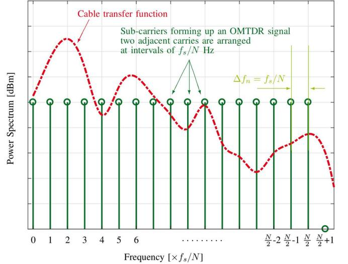
Fig. 2. Positive part of the spectrum of an OMTDR signal  $X(f_n)$  with  $N$  sub-carriers (green) and the cable frequency-domain transfer function (red) defined in the same band as the multi-carrier signal, i.e.,  $f_s/2$  with  $f_s$  being the DAC sampling frequency.
