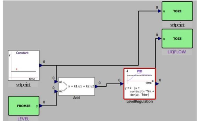
Fig. 4. View of the PI controller sub-model taken from the PEGASE framework.
