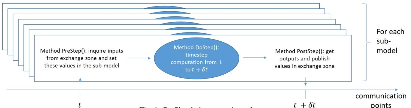
Fig. 1. Co-Simulation execution scheme.
