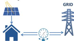
Figure 4: Net metering scheme
