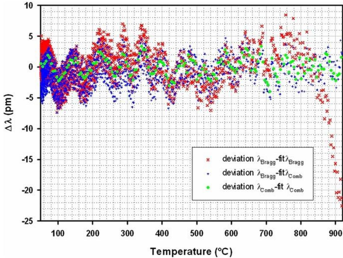
**Figure 7.** Deviations between the experimental Bragg wavelengths with regard to a fifth-order polynomial fitting processed on averaged (blue point, subset averaged every 5  $^{\circ}\text{C}$ ) and non-averaged (red point) data. The green points stand for the error between the averaged data and the polynomial fit computed thereon.
