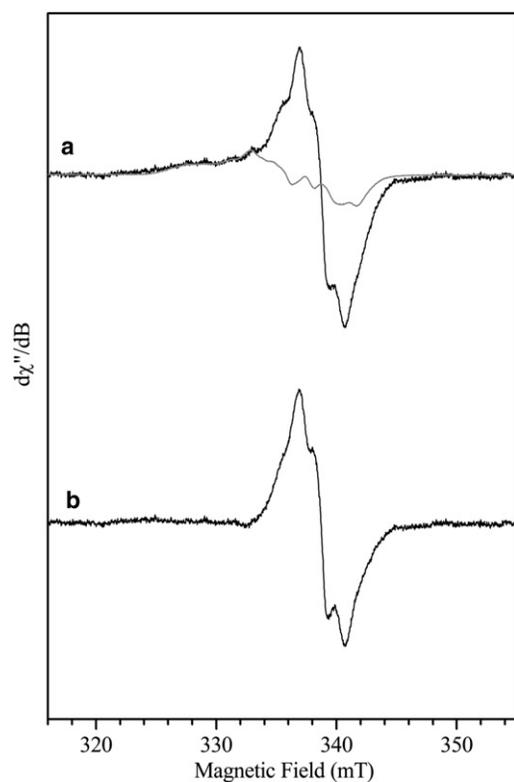
FIGURE 3  $g = 2$  region of the 9 GHz EPR spectra of the 60 ms iNOSoxy + NOHA freeze-quench sample. iNOSoxy/NOHA stopped at 60 ms (black line), scaled spectrum of a prepared iNOSoxy Fe<sup>II</sup>NO sample with NOHA as substrate (gray line) (a); difference spectrum between the last two (b). Measurement parameters: microwave frequency 9.496 GHz, microwave power 1 mW, field modulation amplitude 0.4 mT, temperature 70 K, accumulation 20 scans.
