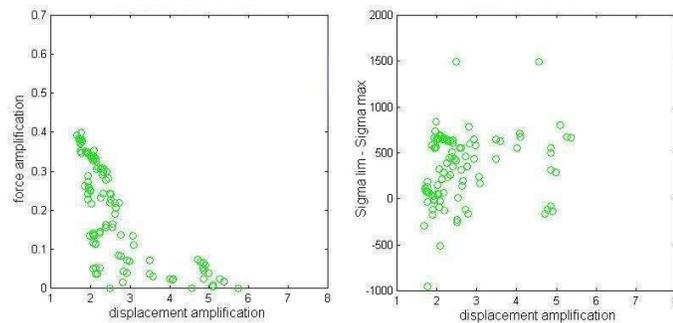
Fig. 12. Pareto front obtained for the optimization with the stress criterion. The structures which have a negative stress criterion are not valid, because  $\sigma_{max} \geq \sigma_{lim}$  (i.e. Von Mises stress greater than yield stress)
