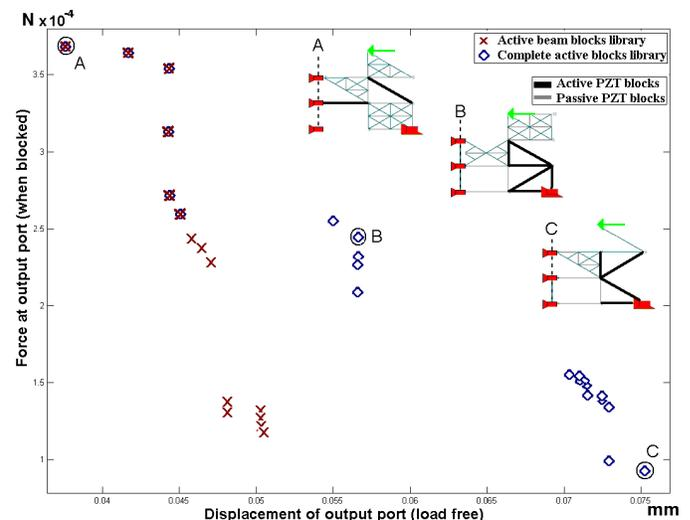
Fig. 14. Pareto graph of piezoelectric compliant microgrippers synthesized using *FlexIn* (half gripper dimensions are 5 mm  $\times$  9 mm, the thickness is 10  $\mu$ m, PZT material is PIC 151 from PI Piezo Ceramic Technology [57], the input voltage is 150 V). A, B and C are selected half-topologies (markers are boundary conditions, arrow is the output displacement optimized).
