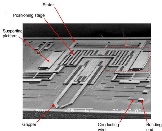
Fig. 6. Single crystal silicon monolithically integrated microgripper, actuated by two linear and one vertical comb actuators [21]. The displacement of the gripper is 5.9  $\mu\text{m}$  under a 50 V driving voltage.
